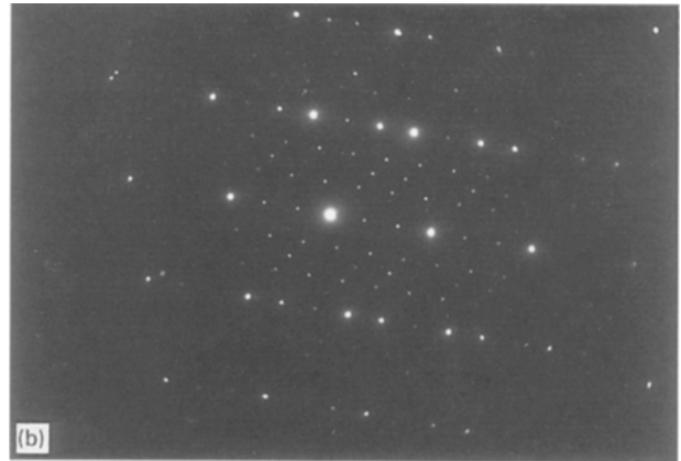
Figure 2 Selected area diffraction patterns showing the crystallography of the \beta , \gamma' and M_{23}X_6 phases for beam direction, B , equal to (a) [1\ 0\ 0]_{\beta} (sample aged for 2 h at 850 °C), and (b) [1\ 1\ 0]_{\gamma'/M_{23}X_6} showing a twinned \gamma' precipitate with one of the twin variants forming a cube-cube orientation relationship with an M_{23}X_6 precipitate (sample aged for 16 h at 850 °C).
